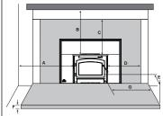
POUR INSTALLATION ET UTILISATION CONFORMÉMENT AUX INSTRUCTIONS DU FABRICANT ET AUX CODES LOCAUX DU BĂTIMENT. HAUTEUR DE PLAFOND MINIMAL: 7PI (2,13m).
